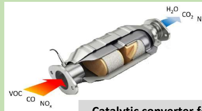
Catalytic converter for gasoline engine
